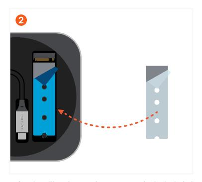
Before installing the SSD, be sure to apply the included thermal tape.
