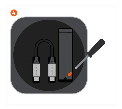
Secure the SSD using the included screw and screwdriver.
