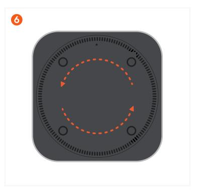
Reattach the cover by turning it counterclockwise until the arrow aligns with the notch and it clicks into place.
