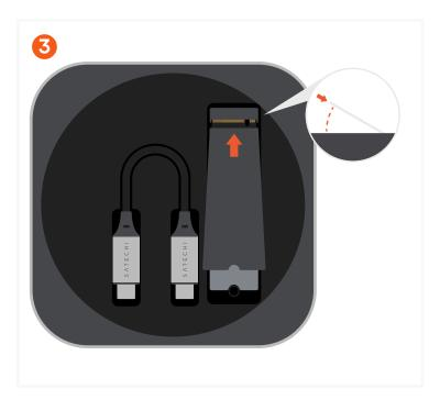
Insert the SSD (not included) at a slight angle and fully seat it in the PCle slot.
