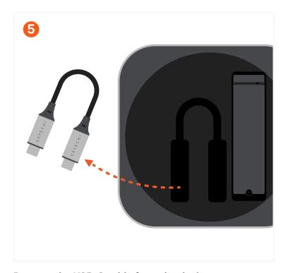
Remove the USB-C cable from the device.
