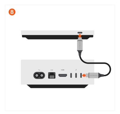
Connect the USB-C cable to the enclosure and then to your computer's USB-C port.
