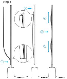
Ensure the exposed wires are inside the lamp base.
