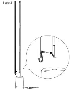
Straighten the silicone strip light. Connect the wires on the silicone strip light to the wires in the port of the lamp base (wires should be connected by color).
