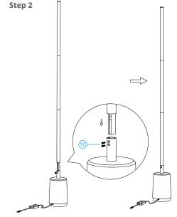
Connecting the lamp pole and lamp base: Insert the connected lamp pole into the lamp base. Use the long screws to secure the final connecting part via the two holes on the base.
