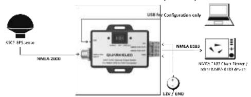
The AS07-N2K can be used out of the box, for instant positional data to your NMEA 2000 bus. Alternatively, the AS07-N2K can be used with the AS07-C Optional Output Switch (pictured above).
