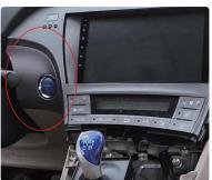
2 Reinstall the center console decorative trim around the radio, then put back the base of the gear shift lever. The installation of the new radio is complete.
