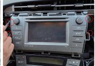
3 Take out the car radio, unplug the wires connected to the original vehicle, and remove the radio.
