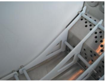
Continue until all three partitions are in place. It will be necessary to push all previously placed components together to make room for the final partition.
