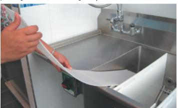
Begin bending the flow guide to the shape of the front rib set, and allow the notches of the flow guide to engage the hooks of the rear rib set.
