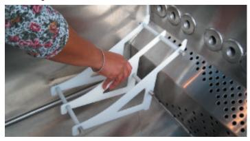
Place the other rear rib sets against the back wall of the sink leaving a finger-size gap between them.
