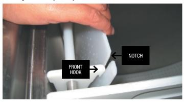
While holding the flow guide against the front rib set, rock the front rib set and the end of the flow guide away from you until the notches in the flow guide engage the hooks of the front rib set.
