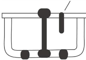
RETENTION BRACKET CLIPPED ON TOTUBE
