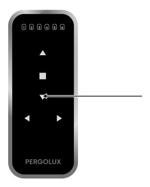
To dim the lights, press and hold the "DOWN" button.
