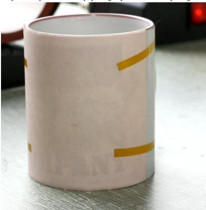
Step 2: Put the cup/mug and the transfer paper into the heat press machine.
