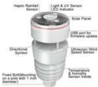
Figure 3 Sensor package assembly components
