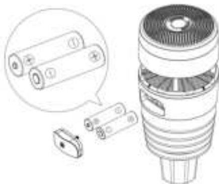
Figure 5 Battery installation diagram
