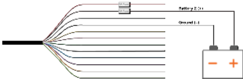
Wired Battery 2 Diagram
