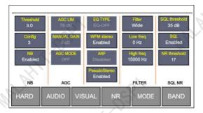
The AUDIO menu allows you to configure various sound characteristics such as filtering, gain, noise reduction, noise cancellation, and squelch.
