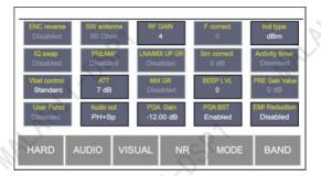
This HARD menu allows you to configure various hardware features such as radio frequency gain, preamplifiers, attenuators, and more. Touch a menu item to select it. If an item has more than two different values, rotate the FREQUENCY knob to toggle between these values. To exit the menu, touch the HARD button again. The menu includes the following items:
