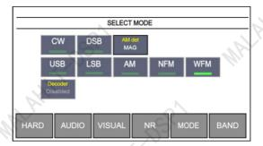
The MODE menu allows you to change the current modulation mode (shown at the top of the screen) and also enables the CW decoder function. Touch a menu item to select it. If an item has more than two different values, rotate the Frequency knob to change between these values. To exit the menu, touch the button again.
