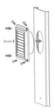
3.Connect the exhaust pipe of the dryer, tighten the screw of the hose clamp to connect the exhaust pipe with the bracket.
