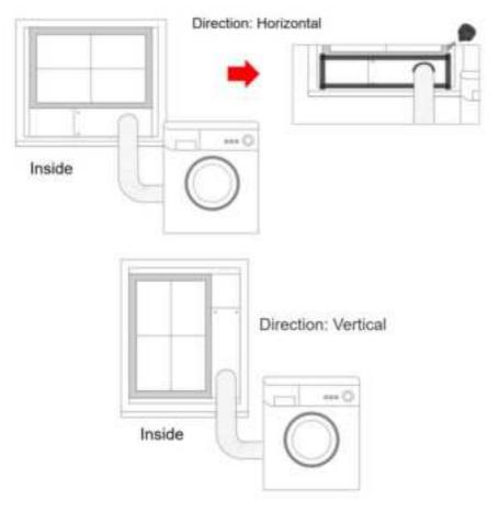
**Attention:**Whether installed vertically or horizontally, make sure the blades are facing down, otherwise water will seep in during rain
