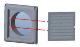
2.Use four screws to secure the shutter to window panel A. Attention: Make sure the fan blades are facing downwards, otherwise water will seep back in when it rains.
