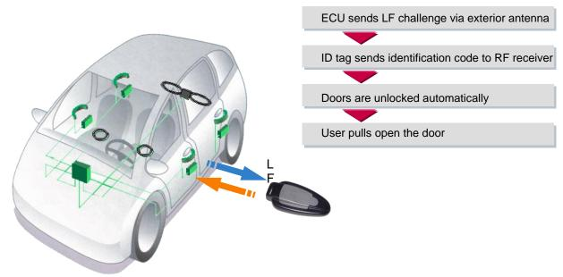
**Figure 1: Principle of Communication**
