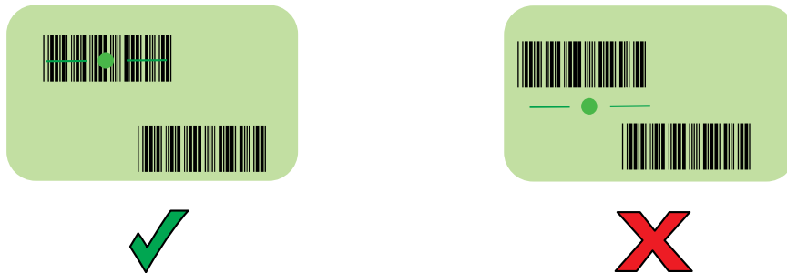
Figure 7 SE55 Aiming for Pick List Mode with Multiple Barcodes
