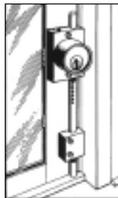
Installation at base of sliding patio door
