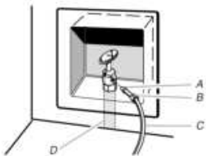
A. Bulb B. Nut C. Copper or PEX tubing (to refrigerator) D. Household supply line (1/2" minimum)
