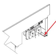
6. Place another washer from kit onto caster, then secure caster to the machine using a locknut from kit and 1/2" wrench.
