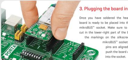
Once you have soldered the headers your board is ready to be placed into the desired mikroBUS™ socket. Make sure to align the cut in the lower-right part of the board with the markings on the silkscreen at the
