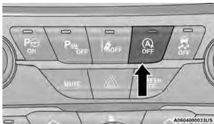
Stop/Start OFF Switch
