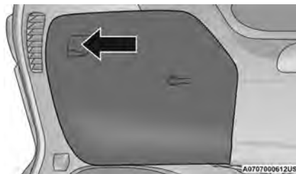
Jacking Equipment Location
