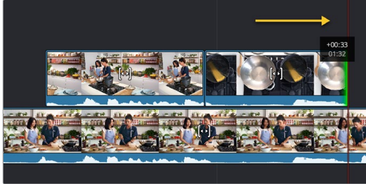
“Painting-on” the next edit by holding down the Camera 7 key and rotating the search dial to the right
