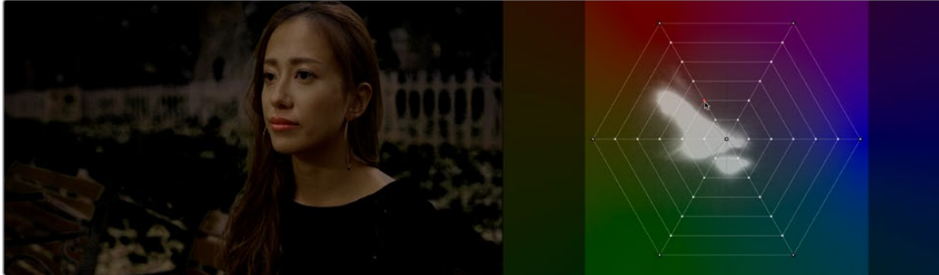
Holding the Option key down while clicking a Color Warper control point shows a preview of affected pixels against black
