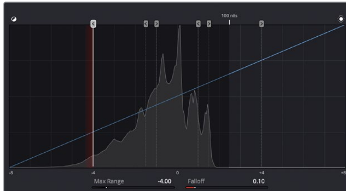
The scale of the Zone graph shows you the shadow and highlight ranges, in stops, relative to 0 representing 18 percent photographic gray
