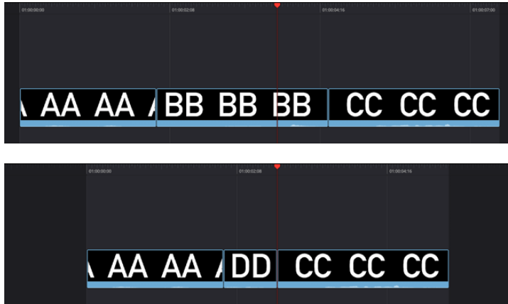
Performing a Ripple Overwrite to substitute an entire clip at the playhead (BB) with the incoming clip (DD)
