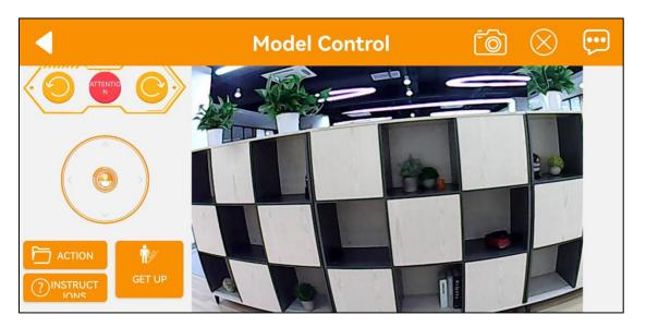
3) The "Model Control" interface consists of two parts. On the left side, you can drag the icon to control the movement of TonyPi Pro. The functions of other icons can refer to the following table:
