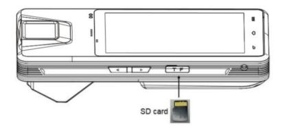
Pull out the TF slot Insert the SD card (Back side up) in the slot Then close the slot
