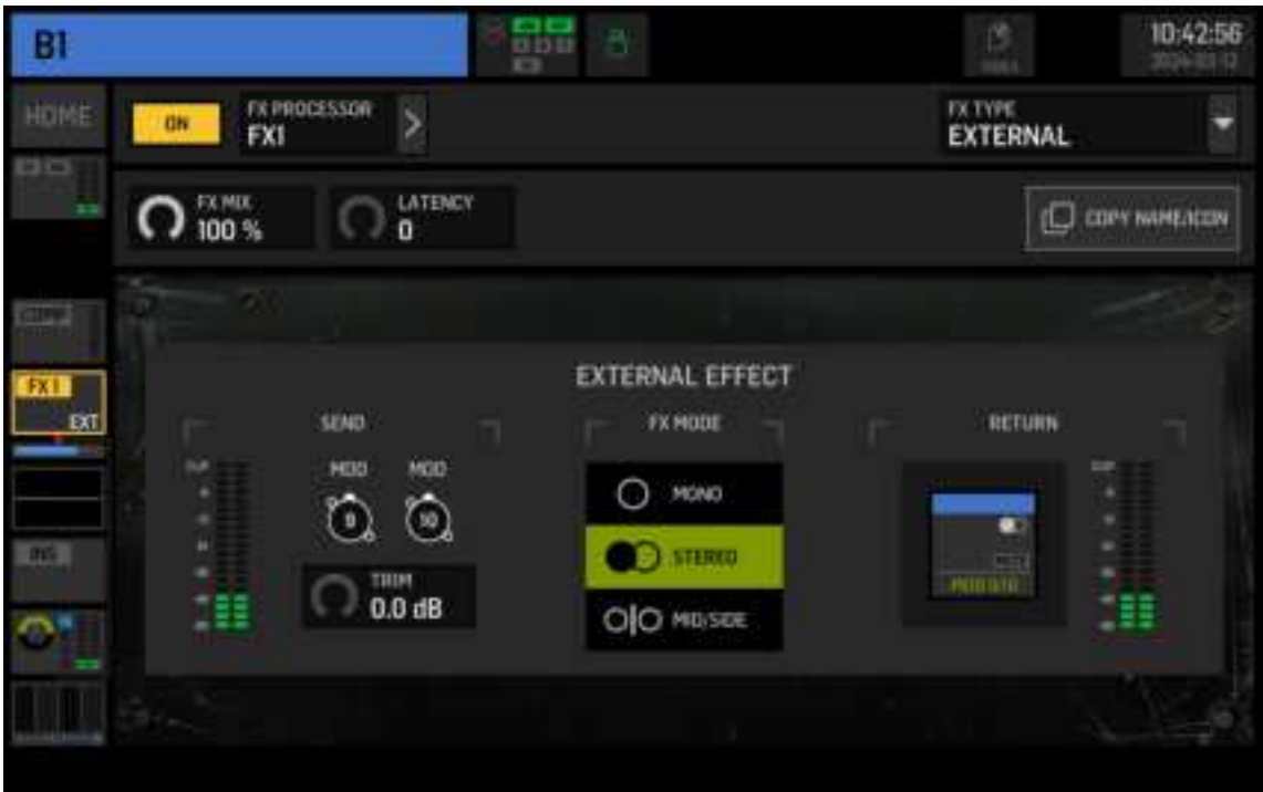
Fig. 7: External loaded as insert point on a bus
