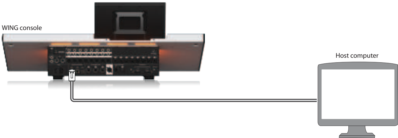
Fig. 1: Direct connection between WING and host computer
