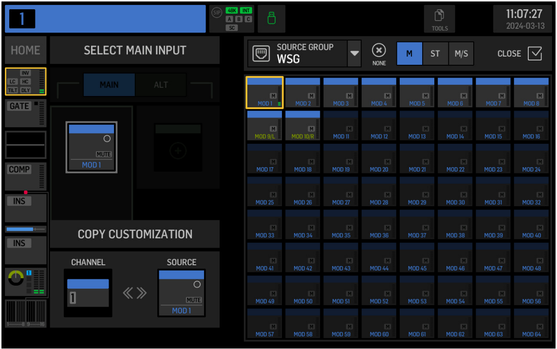
Fig. 6: Assigning SOURCE GROUP WSG to a channel
