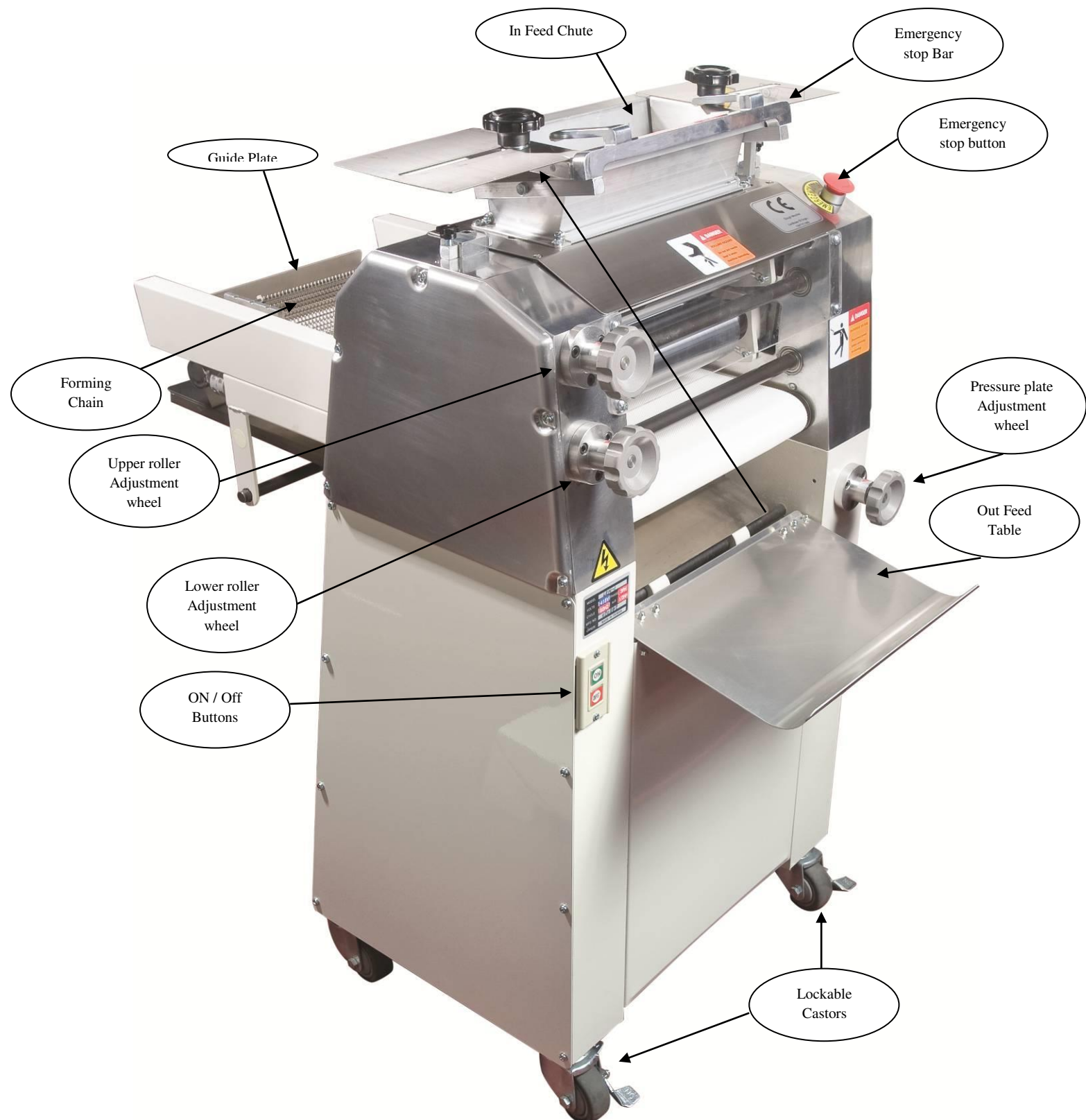
Fig1.2 Main Machine Components
