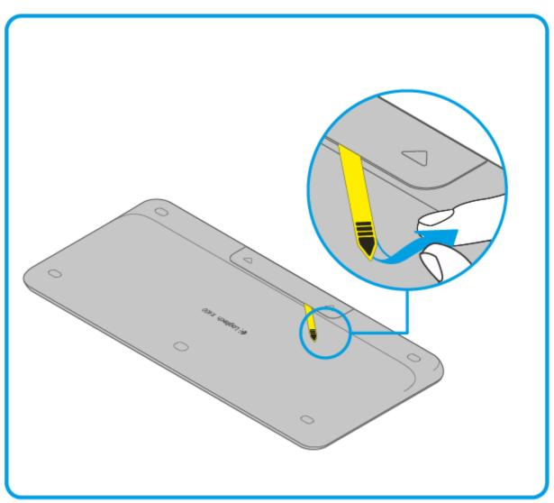
Step 2: Pull to remove the yellow battery tab.
