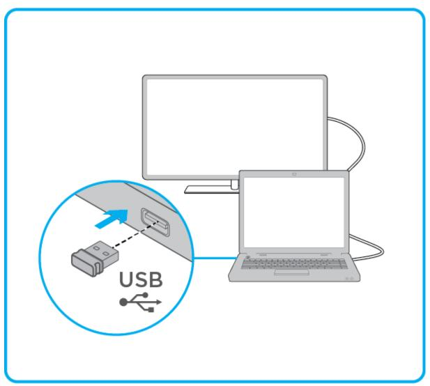
Step 1: Insert the Unifying receiver into a USB port on your computer.
