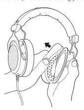
➤ To attach the ear pad, carefully pull the lip over the edge of the housing.
