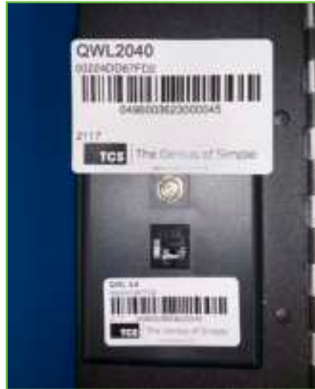
Placement of replacement Gateway label
