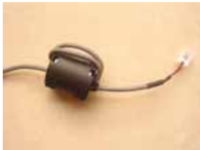
Fig.7.2.6.3 Connection Location of Crystal Connector, Communication Line and Magnetic Ring
