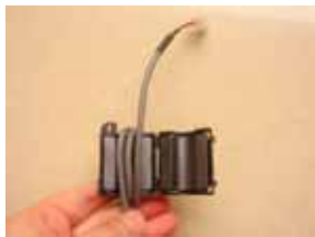
Fig.7.2.6.2 Connection Manner of Crystal Connector, Communication Line and Magnetic Ring
