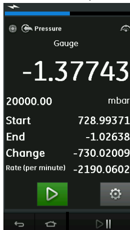
Figure 2-24: Leak Test Example
