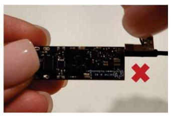
To charge the battery, plug in USB-C while the battery is attached to the SIU. Currently, there's no LED behavior for charging the 10631 battery. LED will remain blue
