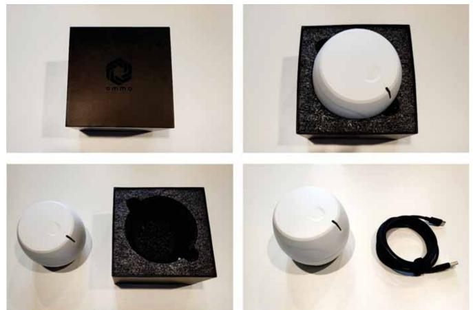
Step 2 | Plug USB-C into the base station and connect to the DPU (computer)
