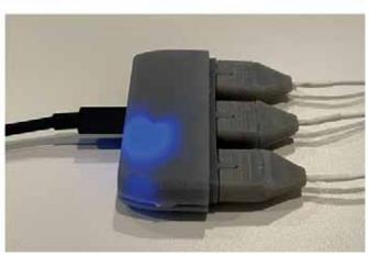
Note: Pictures above shows the device with v5002. For devices with v5004 and higher, LED will show white when plugged in and in idle mode.
