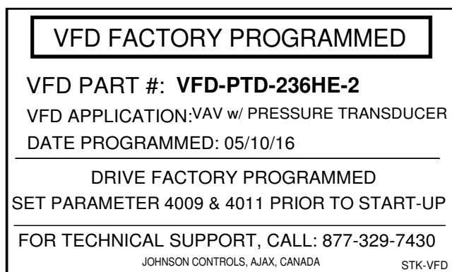
FIGURE 1 - WARNING LABEL ON UNIT/VFD FOR VAV WITH PRESSURE TRANSDUCER
