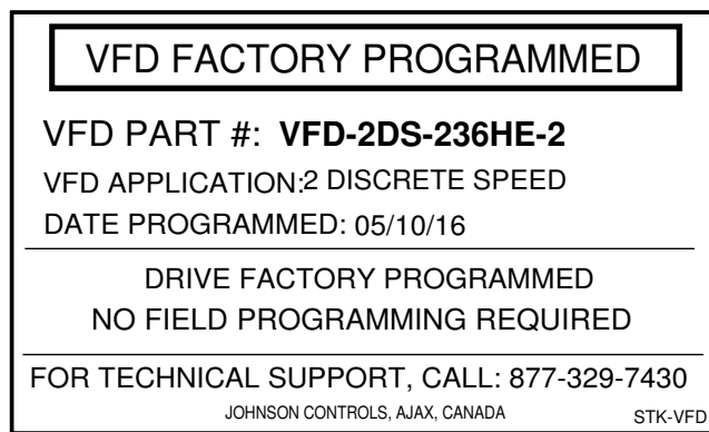
FIGURE 2 - WARNING LABEL ON UNIT/VFD FOR DISCRETE 2 SPEED FAN CONTROL
