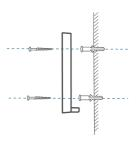
3. Screw the mounting base onto the wall.
