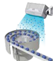
Static elimination in feeder bowls
