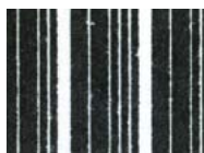
Thick print lines (coated paper)
