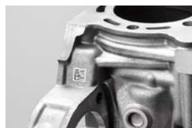
[HIGH-SPEED 2D CODE MARKING] METAL CASTING
