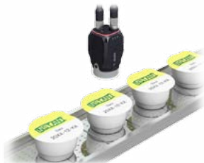
Color detection tool checks printing
