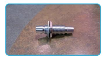
Assemble the return fitting as shown. This includes a double ended barb fitting, low profile nut and white rubber washer.
