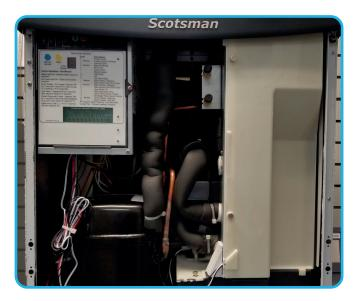
Install the white plastic wall. Sanitize this as well before turning the ice machine on and closing the cover.
