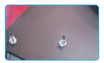
The fittings on the top side of the lid should be completed as shown. Ensure the fitting nuts are tight and prepare to mount the ICEZONE unit.
