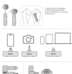
2. Push the selected adapter into the receiver. Connect the receiver to your audio devices, such as a camera, smartphone, tablet, computer, etc.
