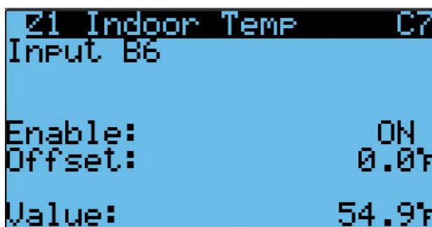
FIGURE 36 Enable/Disable Zone 1 Indoor Temperature Sensor
