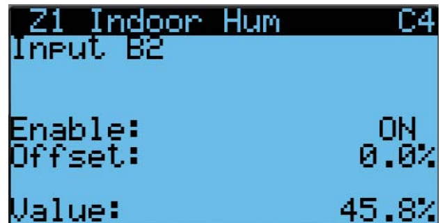
FIGURE 32 Enable/Disable Zone 1 Indoor Humidity Sensor
