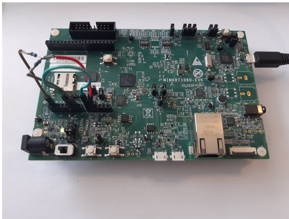
Figure 3. Hardware connection of EVK-MIMXRT1060
