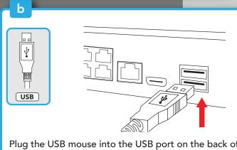
Plug the USB mouse into the USB port on the back of the NVR.  $\label{eq:plug}$
