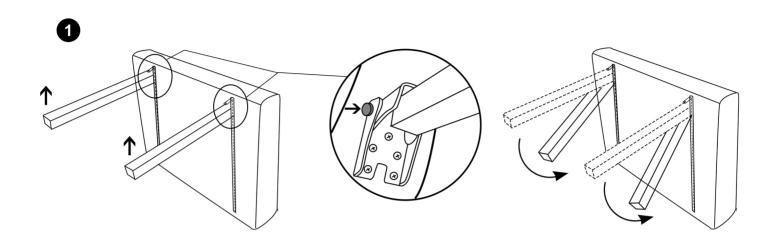
1. There is a round button on the side of the base of the backrest leg. First lift the chair leg up slightly, press the button, and then retract the backrest leg.
