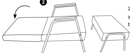
2.After the backrest is completely flattened, you will hear a click and you can adjust the backrest angle back.
