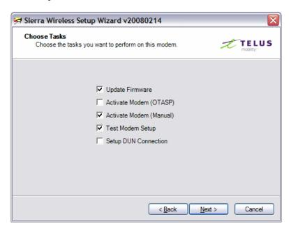
\*NOTE: The Activate modem (OTASP) can be used to automatically pull down the needed information from the network. This is however not recommended as it will not pull down the 1X network settings which are needed to work in those areas where EV-DO coverage is not available.
