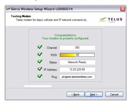
10. At this point the modem is now ready for advanced programming using AceManager. These following steps need to be completed fairly quickly as the modem is on a dynamic IP network and the IP address can change at any time.
