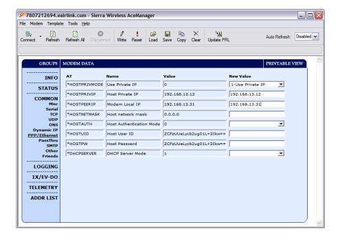
8. Click on Misc in the list on the left. Change the DPORT to 3000. This makes sure that any information sent to the modem from Loggernet on port 6785 will get passed through the Ethernet port and not trapped by the modem.
