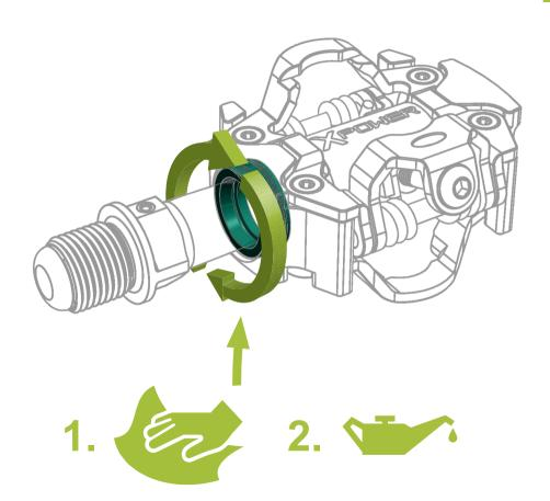
To keep the X-Power pedals running smoothly you don't need to disassemble them. Simply use a dry cloth and wipe away the dirt and debris around the green outer seal.
