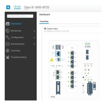
**3.** Once logged into the Local Manager, navigate to Configuration > Services > IOx. For example: Cisco IE3300 10G/IE3400
