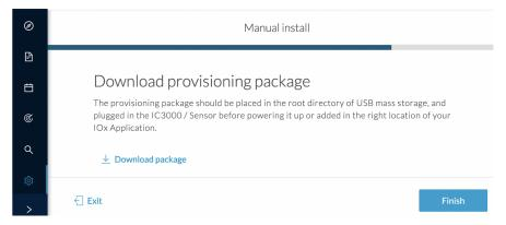
This will download the provisioning package which is a zip archive file with the following name structure: sbs-sensor-config-<serialnumber>.zip (e.g. "sbs-sensor-configFCW23500HDC.zip").
