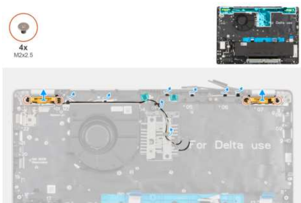
Figure 76. Removing the WLAN antenna module
