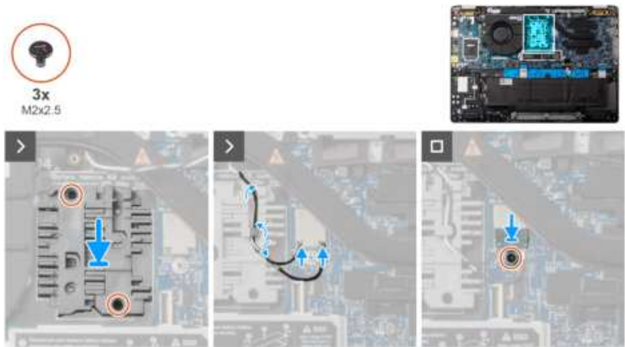
Figure 82. Installing the keyboard filler
