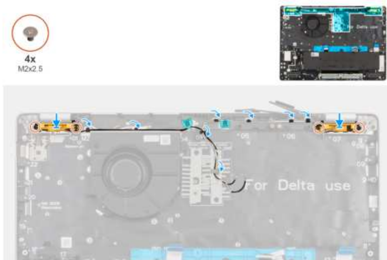
Figure 77. Installing the wireless antenna
