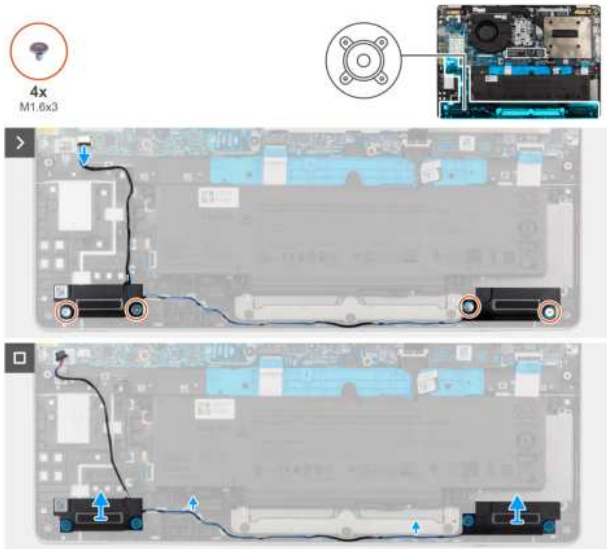
Figure 30. Removing the speakers
