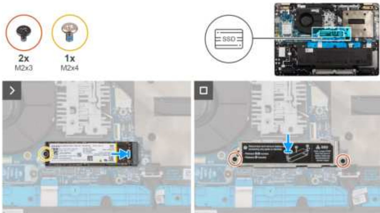
Figure 27. Installing the M.2 2280 SSD
