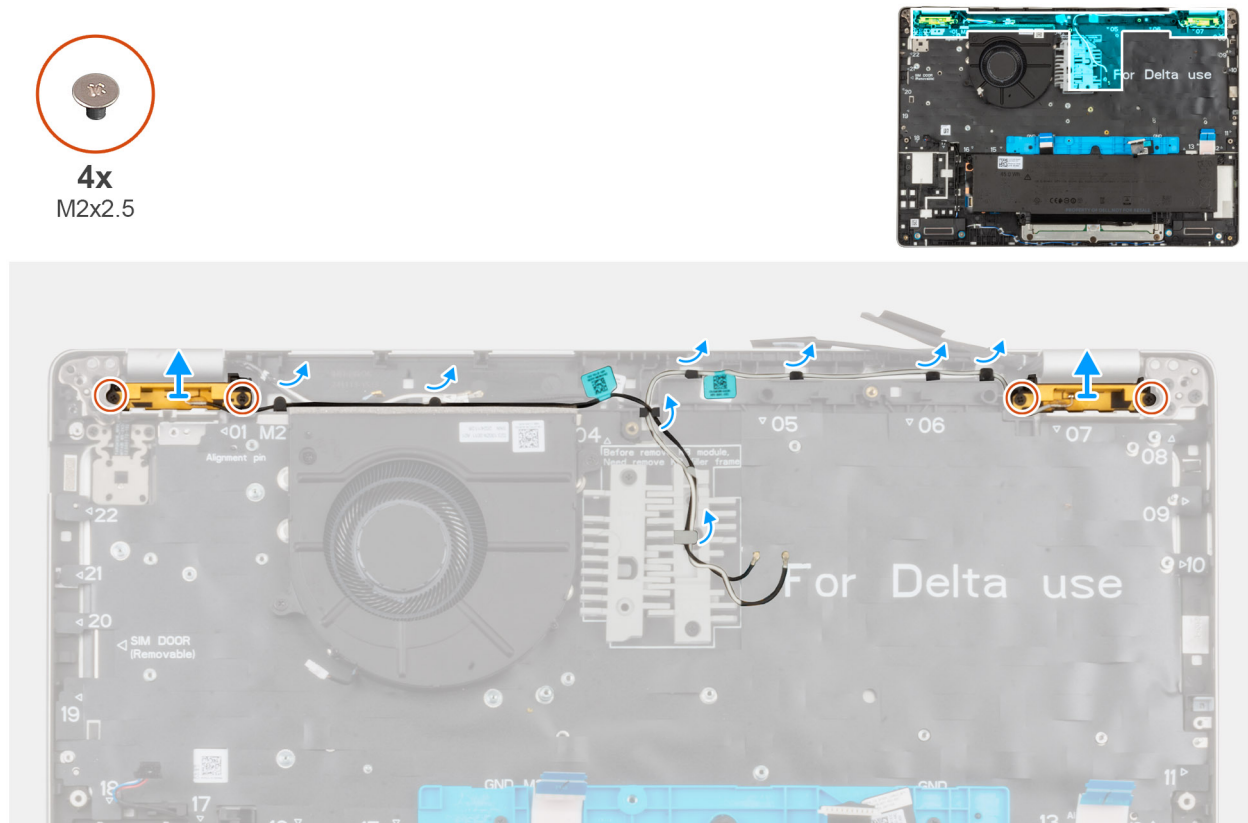
Figure 76. Removing the WLAN antenna module
