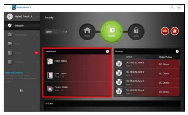
The control panel constantly checks the system for any faults. When fault event exists in the system, the panel Orange LED 3 will turn on. The Panel Status column in Dashboard will change to red, the fault icon will appear on top left corner of the Panel icon to alert the user. Click the panel icon to check the detailed fault information.
