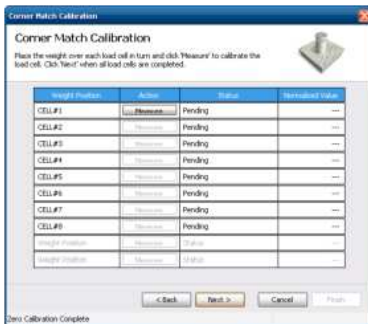
Figure 5-13. Corner Match Calibration Wizard
