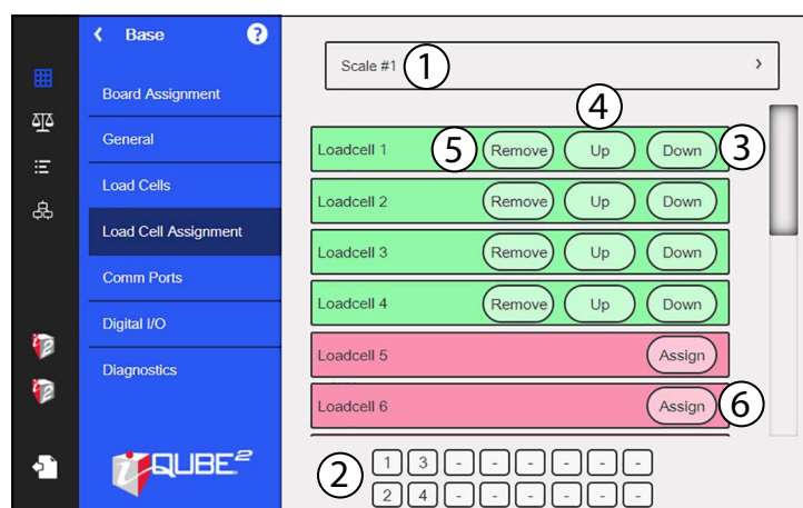
Figure 3-3. Load Cell Assignment Display
