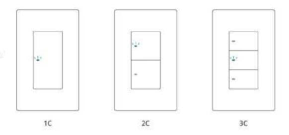
① The device will exit the pairing mode if you do not operate it within 3mins. When you want to enter the pairing mode again, long press the any button on the device for 5 seconds until the signal light "flashes slowly" and release.
