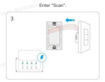
Install the device into the mounting box first, then power it on.
