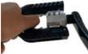
Pull the middle ring away from the bike.
