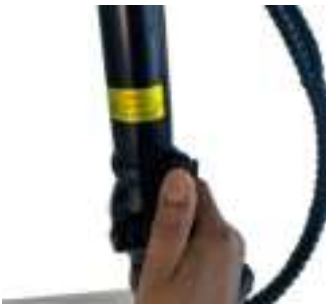
Using your fingers push the latch to the side
